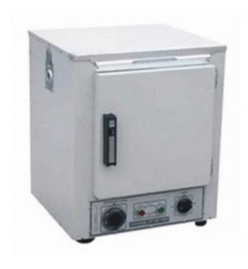
Standard double wall fabrication, Inner chamber made of richly anodized aluminum or highly polished stainless steel sheet. Exterior fabricated out of thick milled steel duly finished in white stoving enamel/Powder coated paint with mat finished Colour combinations. Kanthal wire heating elements provided on three sides to attain quick and uniform heating in range of 5° C to 25 0° Ci 2° C, controlled by capillary type thermostat.
